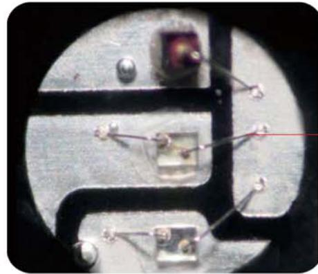
Useing gold wire which has the best electrical and thermal conductivity.
